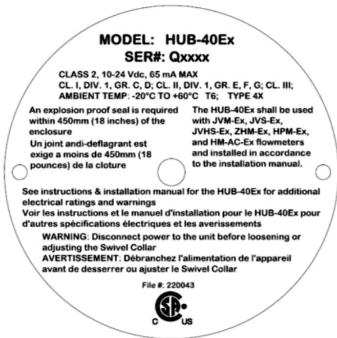
Figure 1: Hazardous Area Certification Tag
